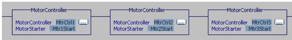
Figure 3 - Three motors controlled in a single rung.
